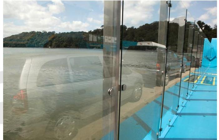
*A glass side has been added to the ferry so passengers can view and appreciate the environment in which they are travelling*
