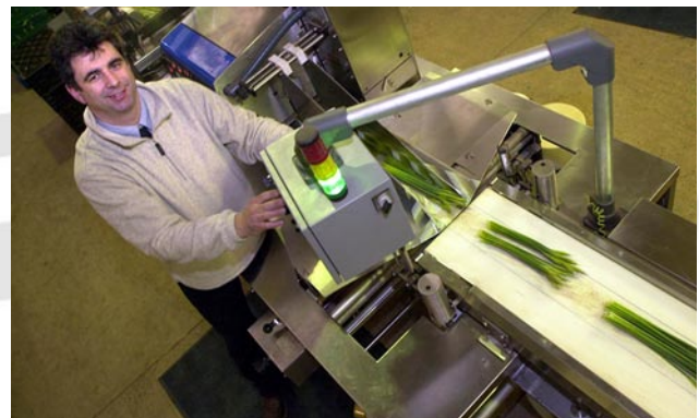
Chris May demonstrates the daffodil flow wrapper at Varfell Farm, Long Rock
